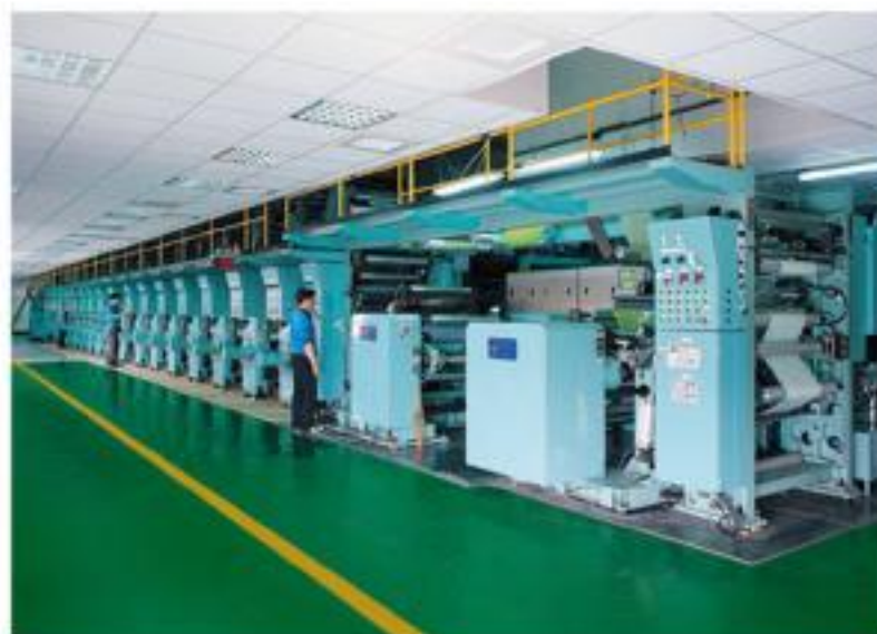
電腦自動對色16色印刷生產線 16-color printing machine with automatic color proofreader
