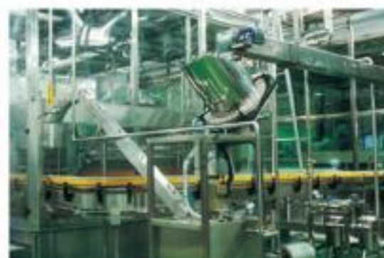
PET耐熱結晶瓶-吹瓶線 Blowing machine for HR PET bottle.
