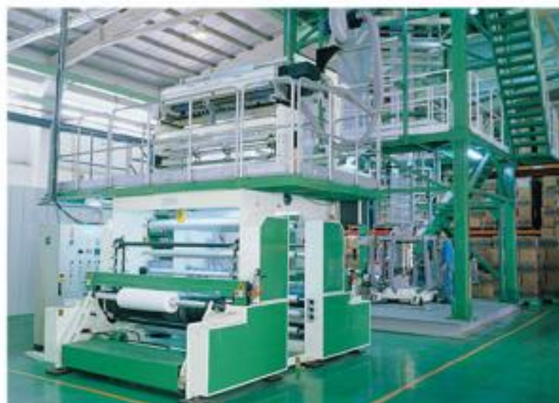
LDPE集合式包裝膜生產線 Production line of LDPE shrinkable film for multipack
