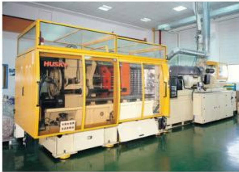
PET耐熱結晶瓶－瓶胚射出設備 High-Speed Preform Injection Machine
